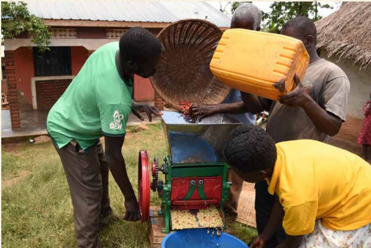
Members of Kwonifur Group (beneficiary farmers of Kyagalanyi) pulping their Arabica coffee in Nyapea Sub-county in Zombo District.
